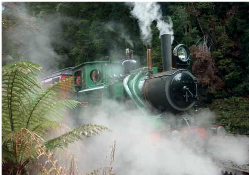
*West Coast Wilderness Railway's Abt 0-4-2T No.5 (North British 24418 of 1938), now fitted with a Lempor exhaust ejector, is seen in action on 27 September 2011.*
