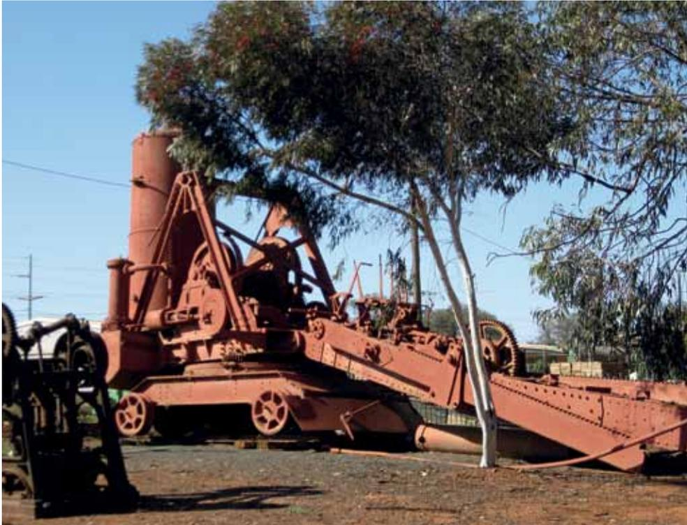
*This unusual vertical-boilered, rail-mounted machine was photographed at Boulder railway station on 24 August 2011. Unfortunately there was no interpretative signage provided, but it is understood that this is a steam navy built by Whittaker Brothers. Can any reader provide details of its origins and purpose?*
