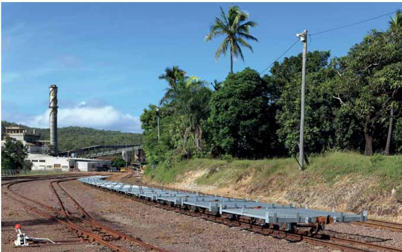
On 4 March 2012, new bin chassis, delivered to the Plane Creek Mill yard, await the fitting of sides and ends in the mill truck shop to be ready for service in the 2012 season.
